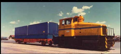
Ambrogio Sr. chose vertical handling and needed craned terminals (Sistema Ambrogio); the system was composed out of three components: the boogie (wheels), the support frame and the loading unit.
